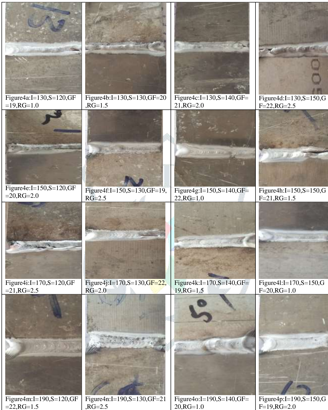
Figure 4: Butt joints welded at different process parameters, I is welding current, S is welding speed, GF is gas flow rate and RG is root gap.
