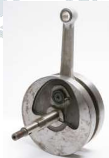
Fig-1 Royal Enfield Bullet 350 cc Crankshaft
