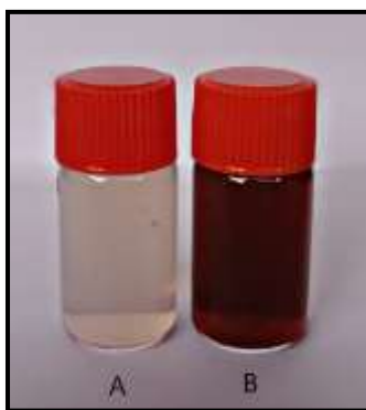
Figure: 1 A: silver nitrate solution with plant extract. B: synthesized silver nanoparticles.
