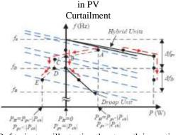
Fig. 12. P=f trajectory illustrating the strength importing state of affairs
