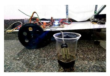
Fig. 9. Testing the Moisture of the Soil
