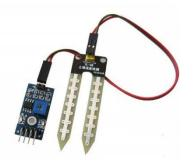
Fig. 6. The Soil Moisture Sensor
