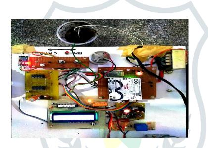
Fig. 10. Testing Soil Moisture, Temperature, Humidity and Illumination System with the Arduino Board
