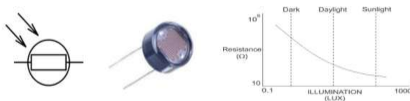
Figure 4: LDR with its characteristics curve
