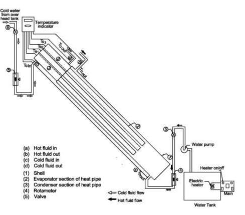
Fig. 1 Experimental setup of gravity-assisted heat pipe heat exchanger.
