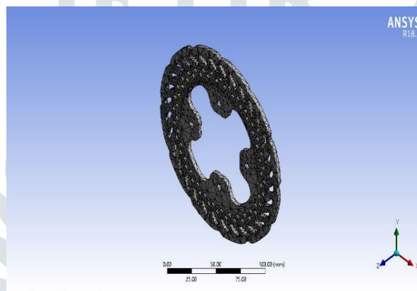
Figure-3: Meshing of brake disc
