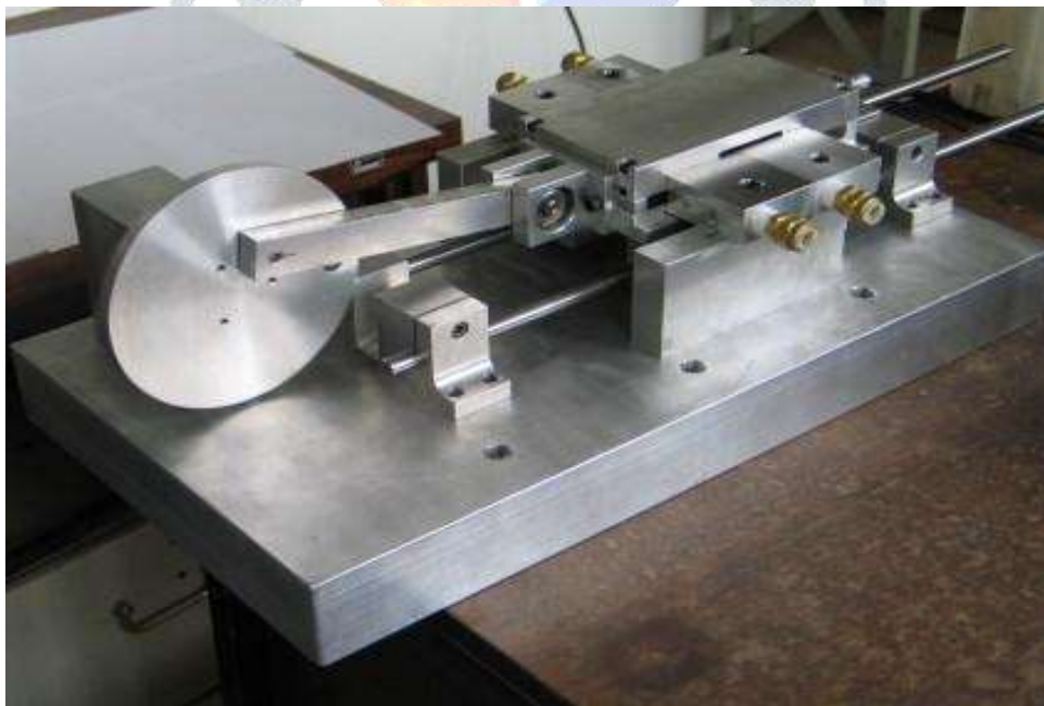
Fig. 4. Picture of the linear reciprocating thermo magnetic motor (global view.)
