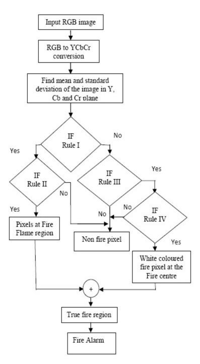
Figure 2. Forest Fire Detection using YCbCr Model
