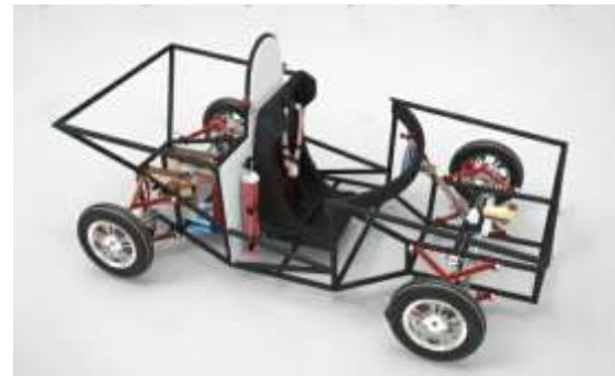
Figure 8 Assembled isometric view prepared in Solidworks and rendered in keyshot 6
