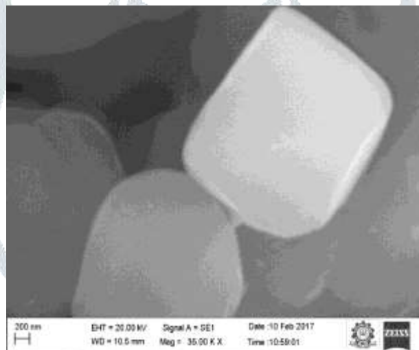
Fig. 5. SEM image of iron oxide nanoparticles synthesized using the extract of Phallusia arabica
