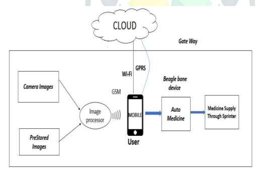
The camera images and the prestored images which are there in beagle bone device are compared and processing is done through the image processor.
