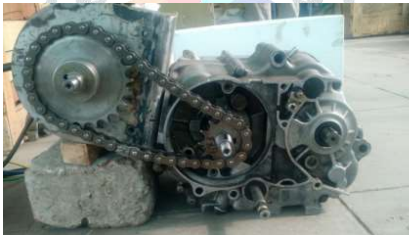
Fig 9: Assembly of gearbox and motor
