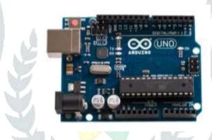
Fig 5: Arduino UNO Board
