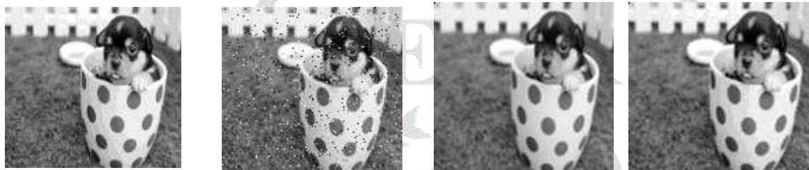
Fig. 1. a)Original Image -Puppy.jpg. b) Gaussian noised. c)median filtered d) BFO based method applied
