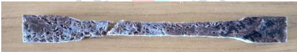
Fig 5.4 tensile tested specimen of fiber strand size 10mm
