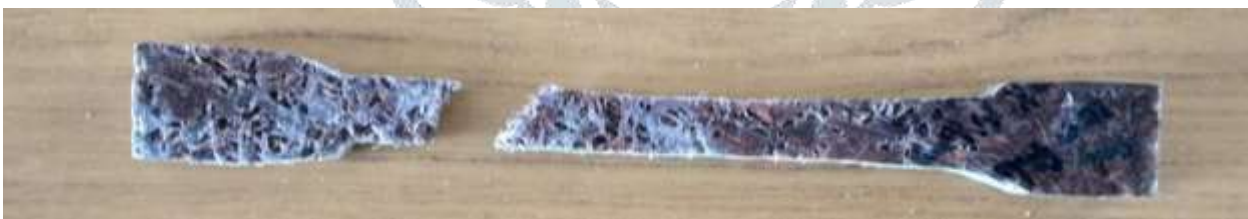
Fig 5.5 tensile tested specimen of fiber strand size 30mm
