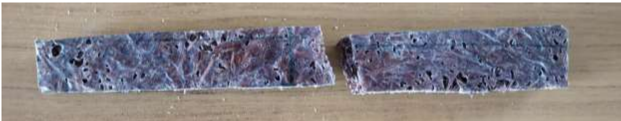
Fig 5.2 flexure tested specimen of fiber strand size 30mm
