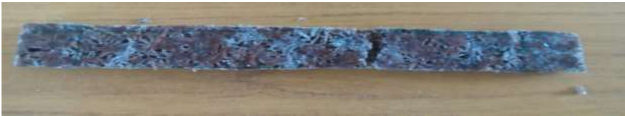
Fig 5.1 flexure tested specimen of fiber strand size 10mm
