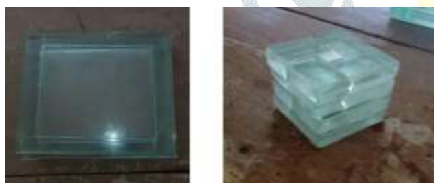
4.2. Tensile and flexural moulds 4.2. Compression moulds
