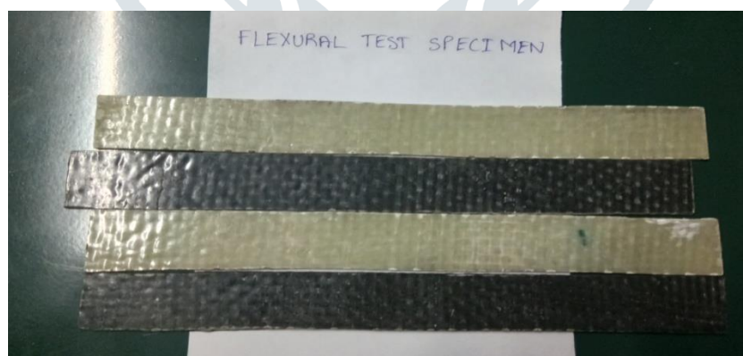
Fig.2 Flexural test specimen
