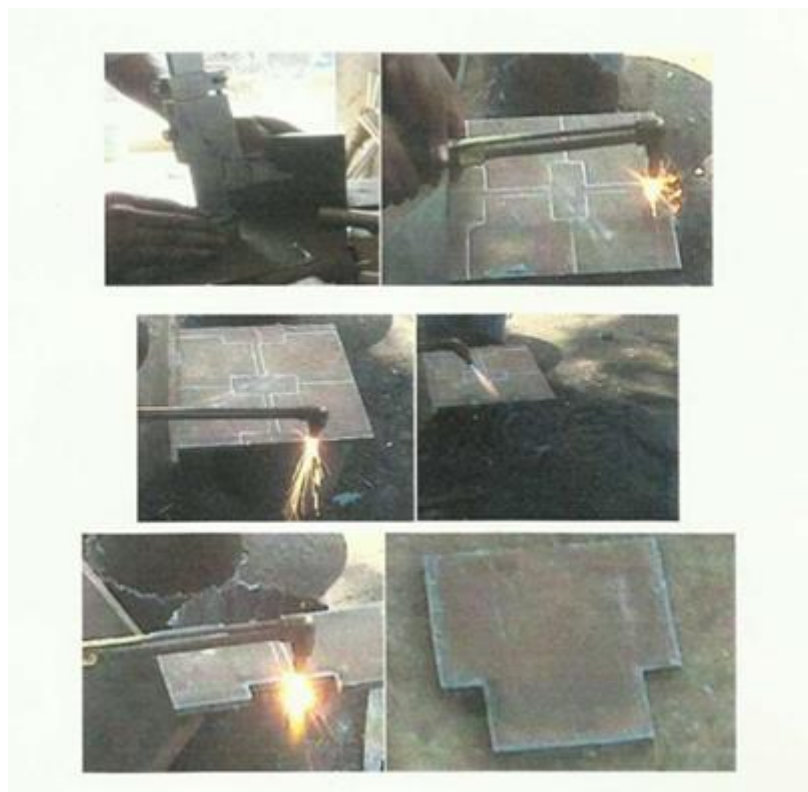
Figure 4: Marking and Plate cutting
