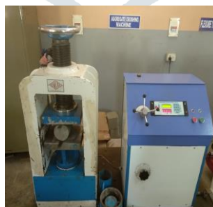
Figure 5.1: Cylinder under split tensile test
