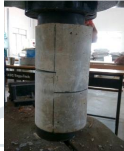
Figure 5.2: Cylinder under shear test
