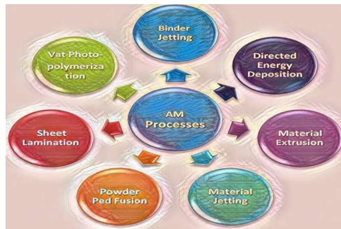
Fig.2. Types of printing technologies
