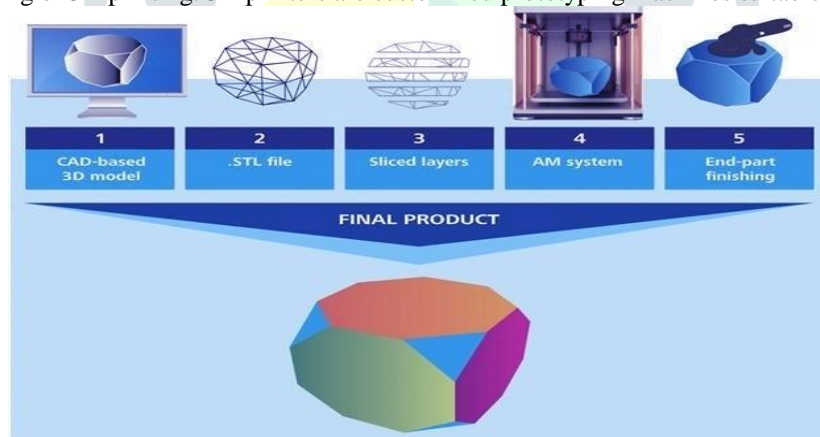
Fig.1. Process done in additive manufacturing.
