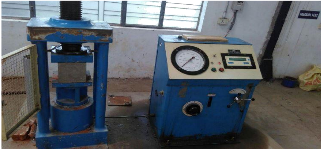
Fig. 8: Compressive strength test
