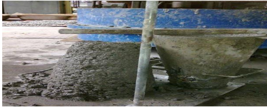
Fig. 5: Workability test conducted in lab
