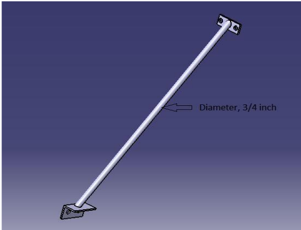
Fig. 5 CAD model of Tubular Side Member
