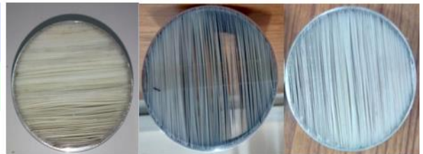
Fig 4: Parallel plate stacks prepared for testing with different porosity ratios
