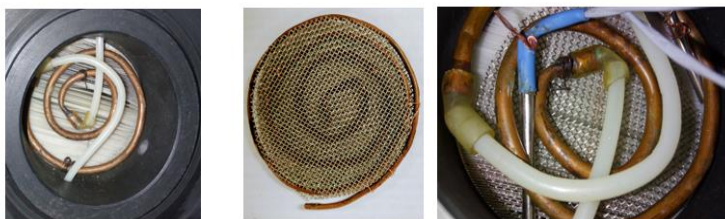
Fig 3: Modified heat exchangers with copper mesh attached to both hot and cold heat exchangers
