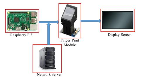
Figure-2: Block diagram of proposed biometric digital transaction system
