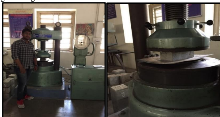
Figure 5 Setup of compressive strength testing of cement brick (At BVM Engineering College Testing Laboratory, Vallabh Vidhyanagar, Gujarat)
