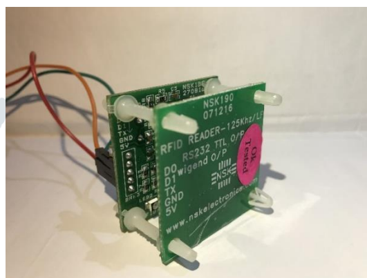
Fig 8.2: RFID Reader is used to detect the vehicle's data.
