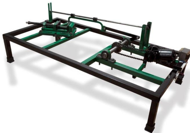
Fig.4 Automatic Motorized Hacksaw Machine with Adjustable Fixture
