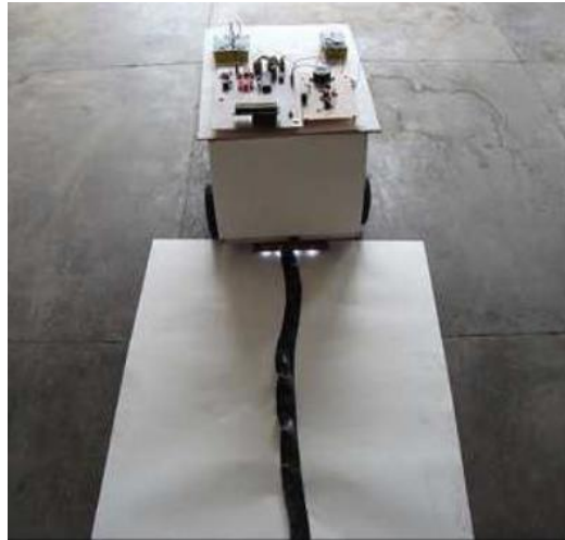
Fig. 6 line following AGV [15]
