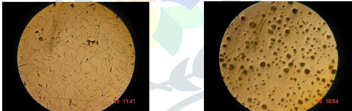
Fig 1.2 Microstructure of gray and ductile iron
