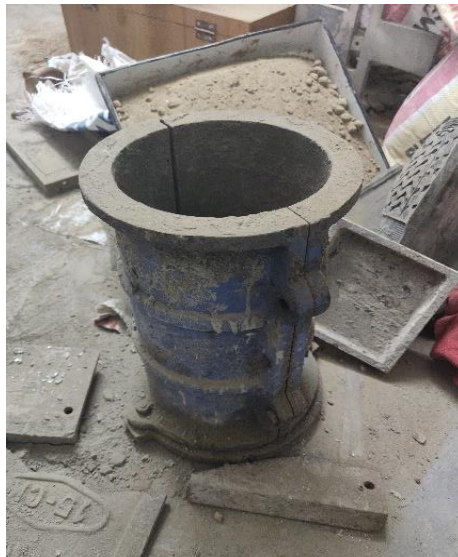
Figure 3. 6: Cylinder (d=150mm, h=300mm) (LPU Concrete Lab)
