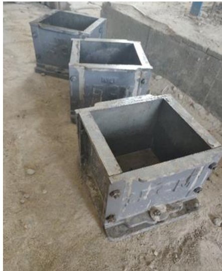
Figure 3. 4: Cube of size (150mm × 150mm × 150mm) (LPU Concrete Lab)
