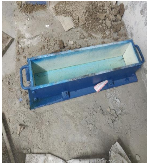
Figure 3. 8: Beam of size (100mm×100mm×500mm) (LPU Concrete Lab)
