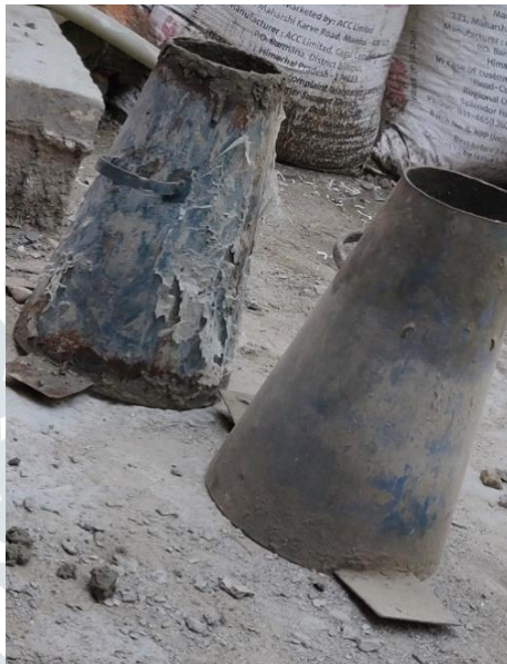
Figure 3. 10: Slump Cone (D=200mm, d=100mm, h=300mm) (LPU Concrete Lab)
