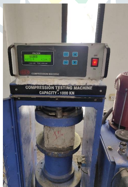
Figure 3. 3: Compressive Strength Testing of a Sample (LPU Concrete Lab)
