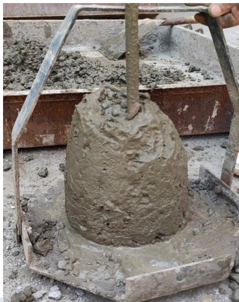
Figure 3. 9: Measuring of Slump (LPU Concrete Lab)
