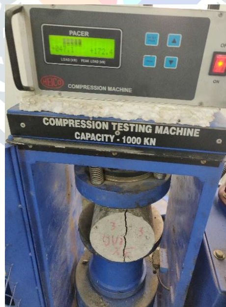
Figure 3. 5: Tensile Strength Testing of a Sample (LPU Concrete Lab)
