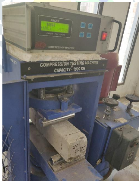
Figure 3. 7: Compressive Strength Testing of a Sample (LPU Concrete Lab)
