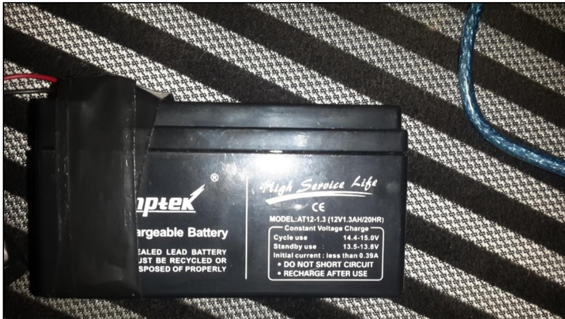
Fig 4: Lead Acid Batteries 14v
