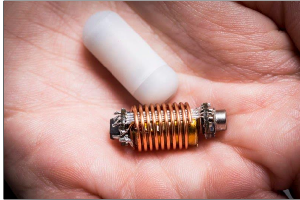
Figure 11: Ingestible electronic capsule
