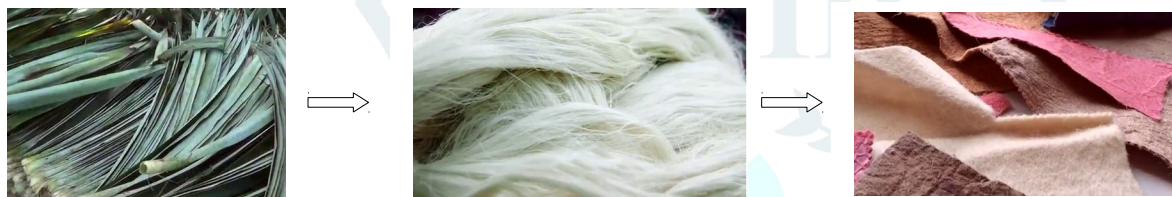
Fig.4 - Leaves to fiber then fiber to artificial leather
