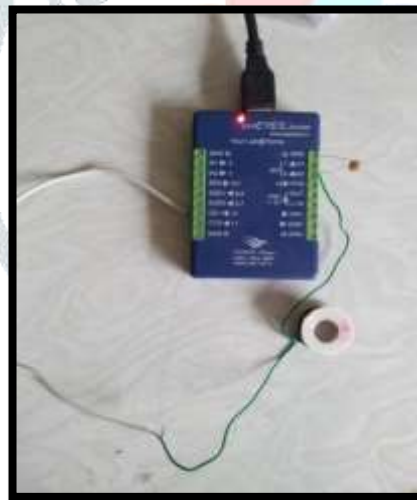
Figure 12: LC series circuit actual connection
