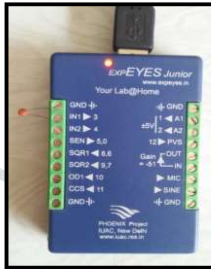
Figure 23: Actual Connection for C measurement
