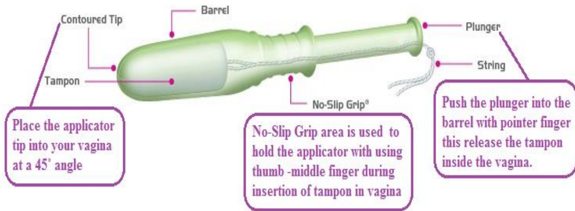
Figure.02: Structure of Tampon with plastic applicator
