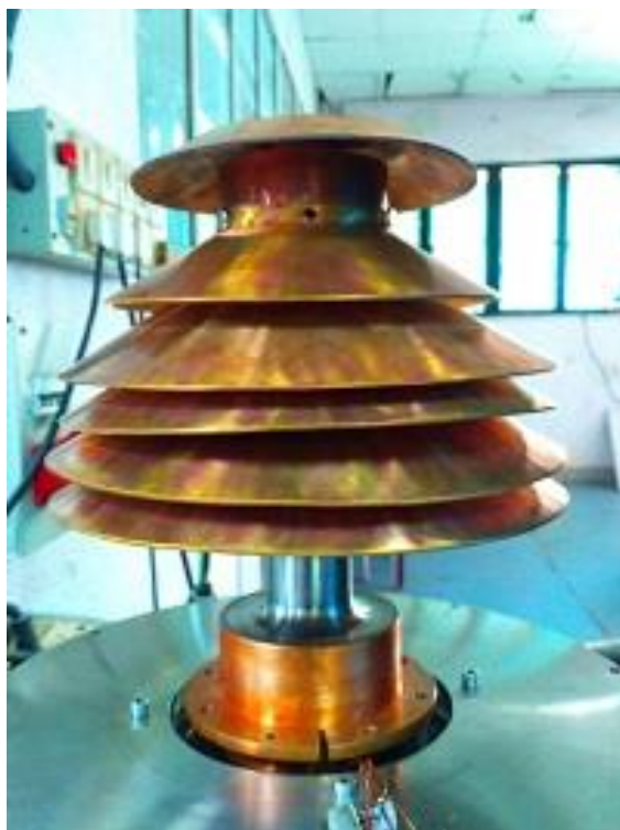
Fig.3 Full section of cryopanel mounted on cryohead
