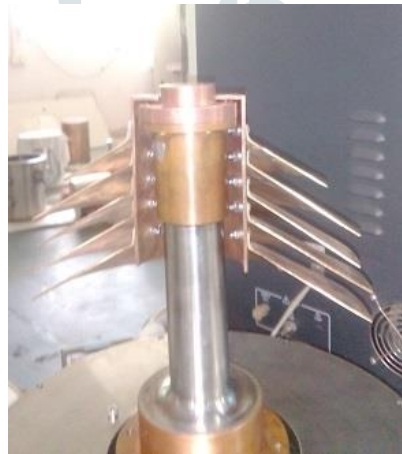
Fig.2 Cut section mounted on cryohead
