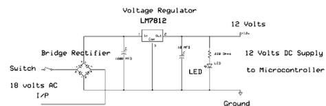
From the above circuit diagram, we can see that the 18v AC is being converted to 18V pulsating DC which is in turn converted to smooth DC with the help of the Capacitor. This 18V Smooth DC is converted to 12V DC by the Voltage Regulator 7812. At the output of the regulator, we get some spikes which are not desirable. These spikes are removed with the help of another capacitor used. We can get 12V Steady DC at the output terminal which can be indicated if the LED glows.
