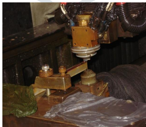
Figure 2 Set-up for Wire Cut Electron Discharge Machining
