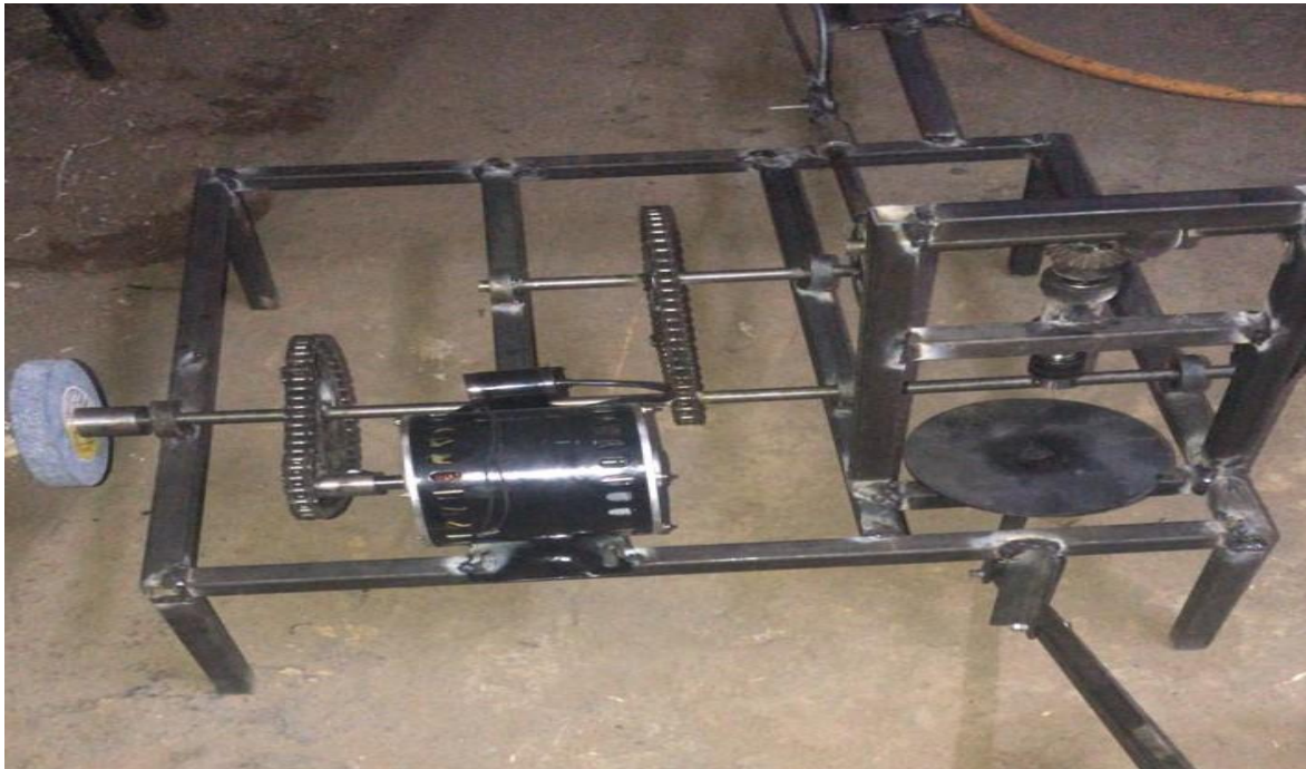
Fig 1 : Fabrication of Multipurpose machine
