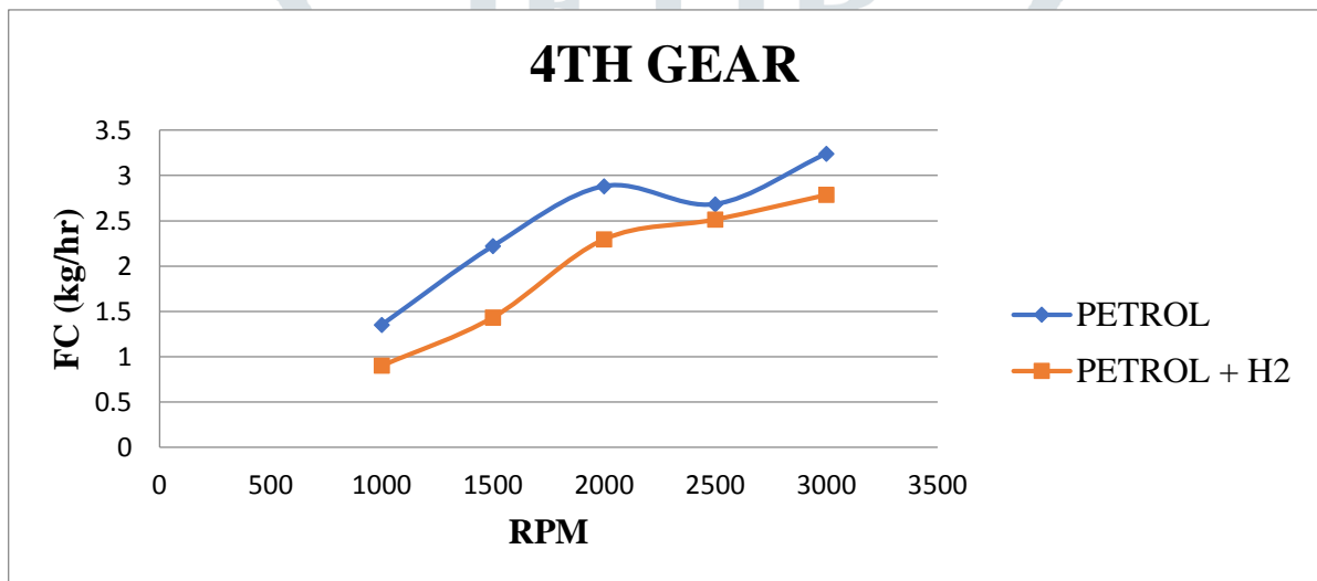
Figure 3.5: RPM Vs. Fuel Consumption for 4 th Gear
