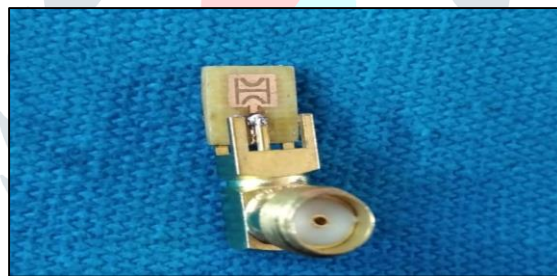
Fig. 8: Dual band microstrip patch antenna with SMA connector
