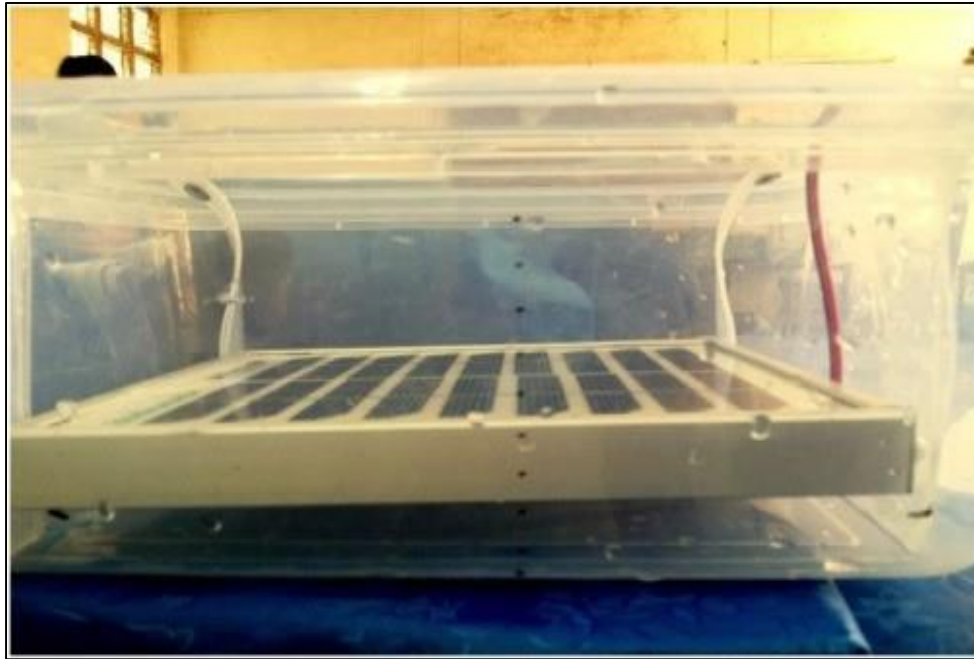
Fig 16:- Panel immersed in water[17].
