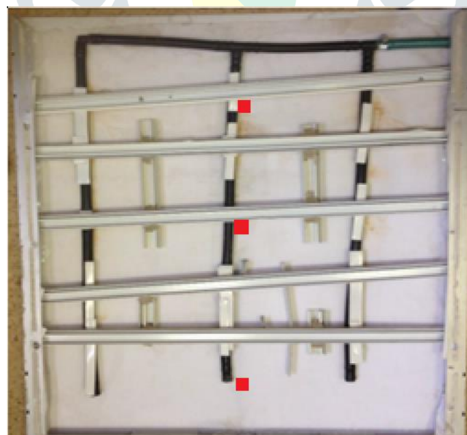
Fig. 19:- The configuration of cloth and pipes on the back of the cooled PV panel.[14]
