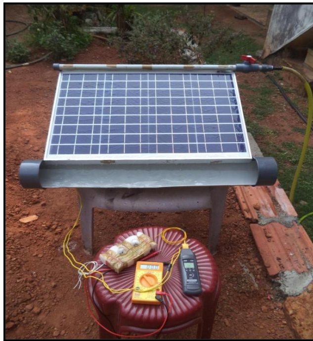
Fig. 14:- With free front flow cooling [12].
