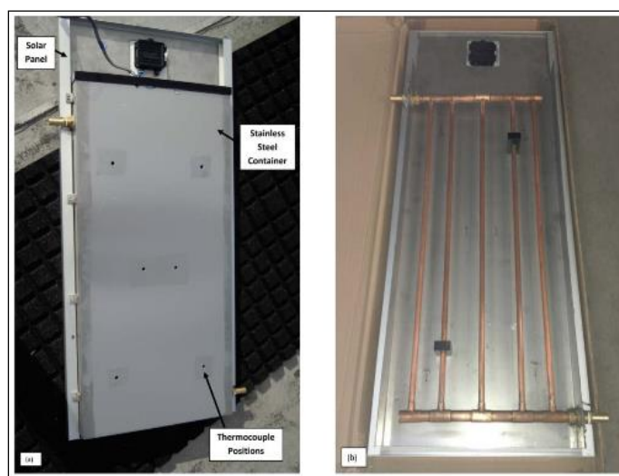
Figure: 8: (a) sealed container (b) pipe network in position in container [17]
