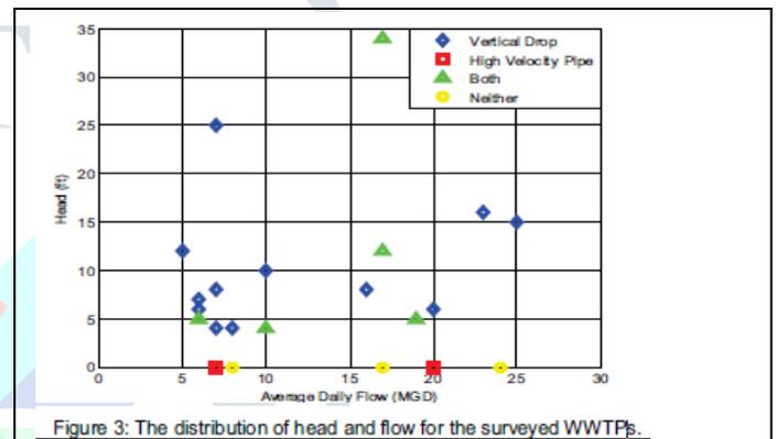
Figure 3: The distribution of head and flow for the surveyed WWTPs.
