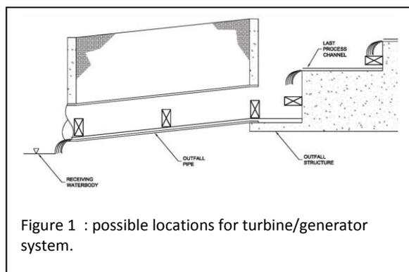
Figure 1 : possible locations for turbine/generator system.
