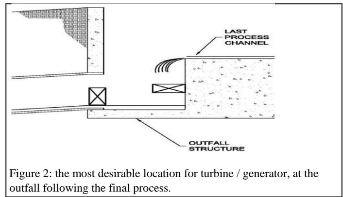
Figure 2: the most desirable location for turbine / generator, at the outfall following the final process.
