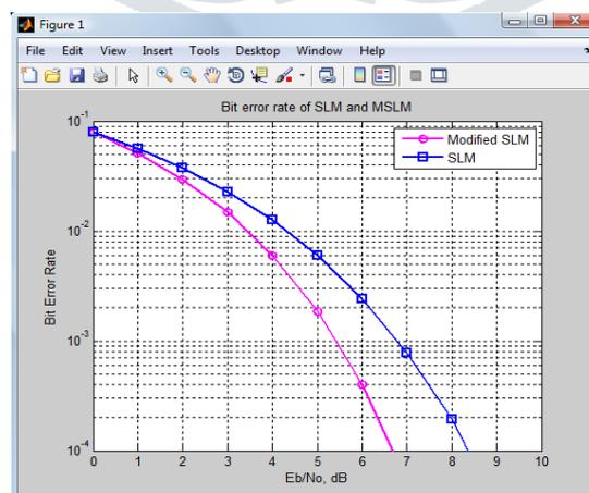
Fig 5 BER Performance of SLM, and MSLM
