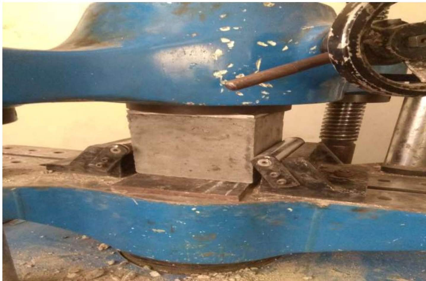
Fig. Compressive strength test of cubes
