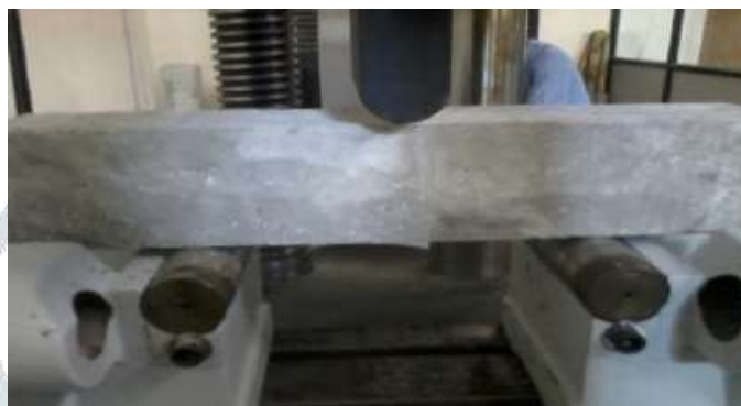
Figure 6: Testing of Beam Specimen
