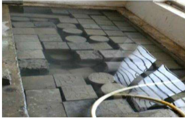
Figure 3: Curing of Casted Specimens
