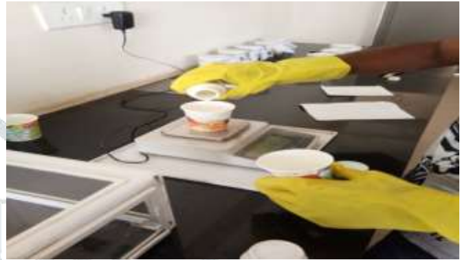
Figure10:- Weighing of Resin and Fibers for Volume Fraction
