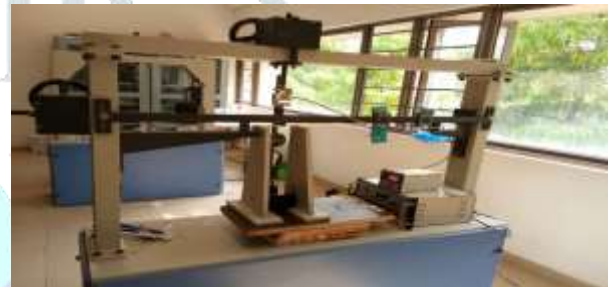
Figure 15:- Deflection Set up
