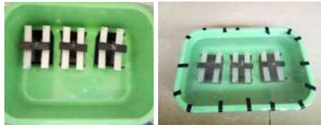
Figure 14:- Specimens Submerged in Sea Water
